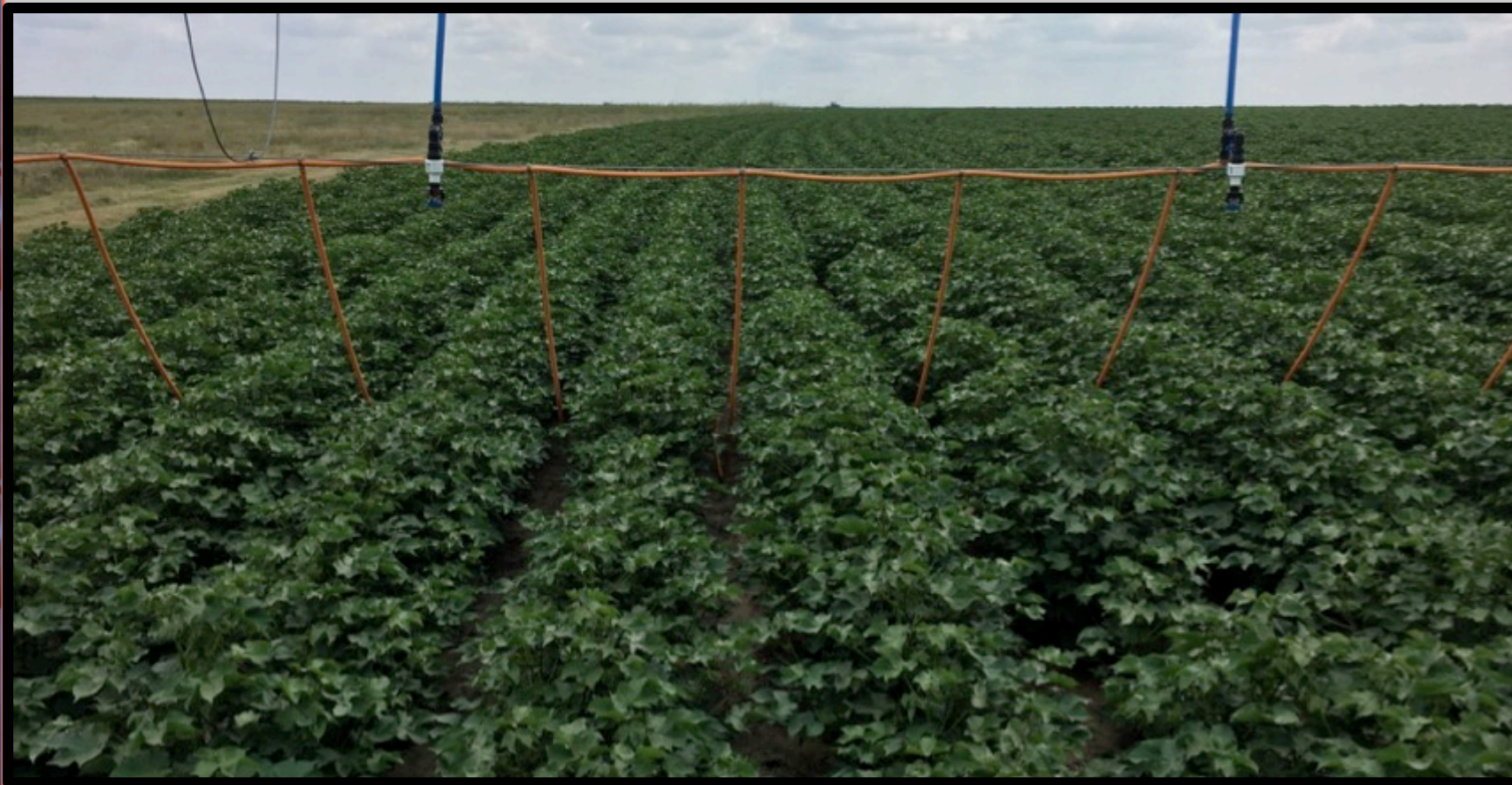
Cotton Mid Season Watering Low-Line System 200 GPM-125 ACRE
